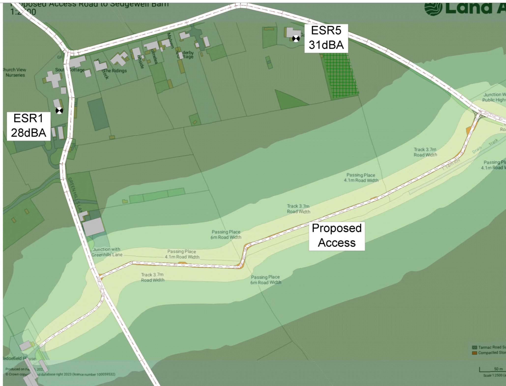
Figure 4: Road Traffic Noise Level - Night-time Peak (dB LAeq,1h) (4m receptor height)
